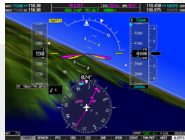
TCAS/TAS/TIS traffic technologies depict targets in 3-D perspective, so you can visually gauge how high and how close they are. Plus, the familiar color- and shape-cued TCAS symbology grows larger as it gets nearer – making traffic conflicts easier to see and identify.
